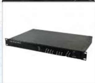
1U solid-state computer boasts 250 I/O points and battery backup
