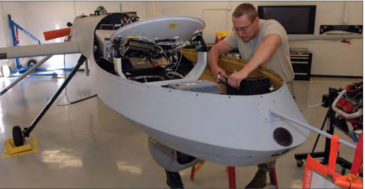
Figure 1 Predator MQ-1 UAVs are packed with electronics. Platforms include day/night Full Motion Video sensors, Signals Intelligence (SIGINT) and Synthetic Aperture Radar (SAR) sensor payload, avionics and data links.
