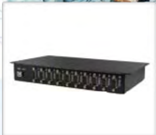
10-port USB adapter designed to meet IEC 60601-1 medical isolation standard
