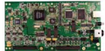
DT9832A — Embedded, Isolated, Simultaneous, 2MHz A/D per channel
